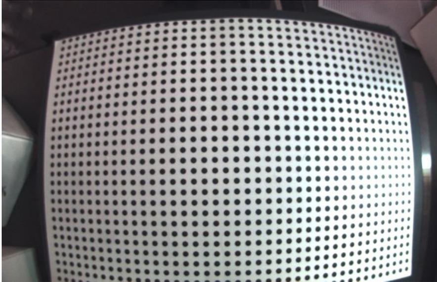
Finally we used a [1/3" format 2.5mm lens](#). This lens format matches the sensor size and therefore it has maximum compatibility with the camera. There is no vignetting shown and the field of view will be at the maximum possible for the lens.
