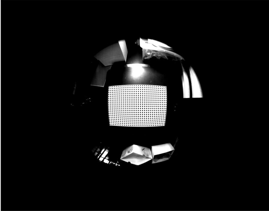
Next up we used an 8mm 1/1.8" format C-Mount lens and a 12mm  $\frac{2}{3}$ " format C-Mount lens.
